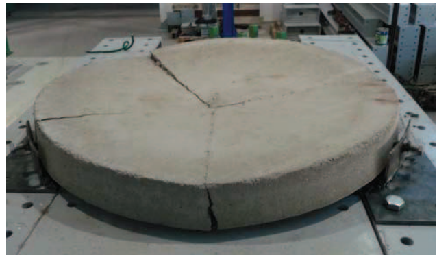
Figure 1. The overall view of an example of the plate after the experimental test. In this case the total damage of the plate has been produced due to the impact of 40 kg weight from 1 m.
